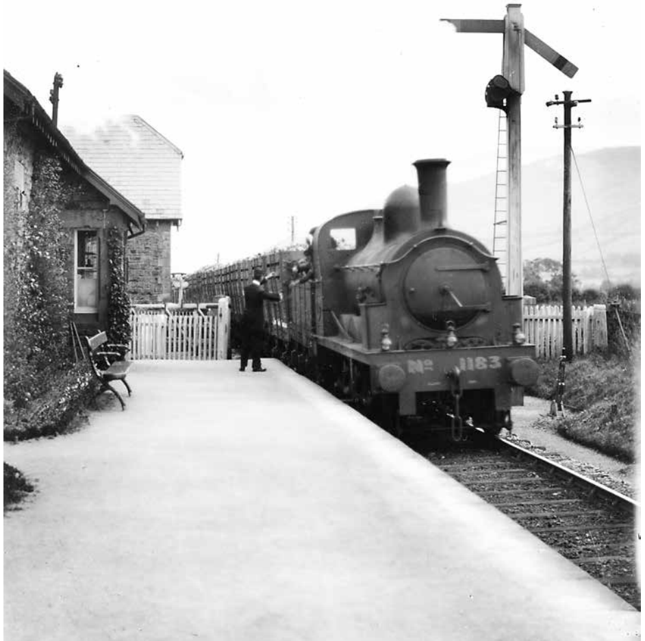
NER 1001 class No 1183 trundles slowly into Embleton station in order to facilitate the exchange of tokens. The visible portion of the train appears to consist of NER Diagram R5 coke wagons. The history of these vehicles was extensively documented in an article by Richard Lacey which appeared in the CRA Journal Vol 8 No 12.
