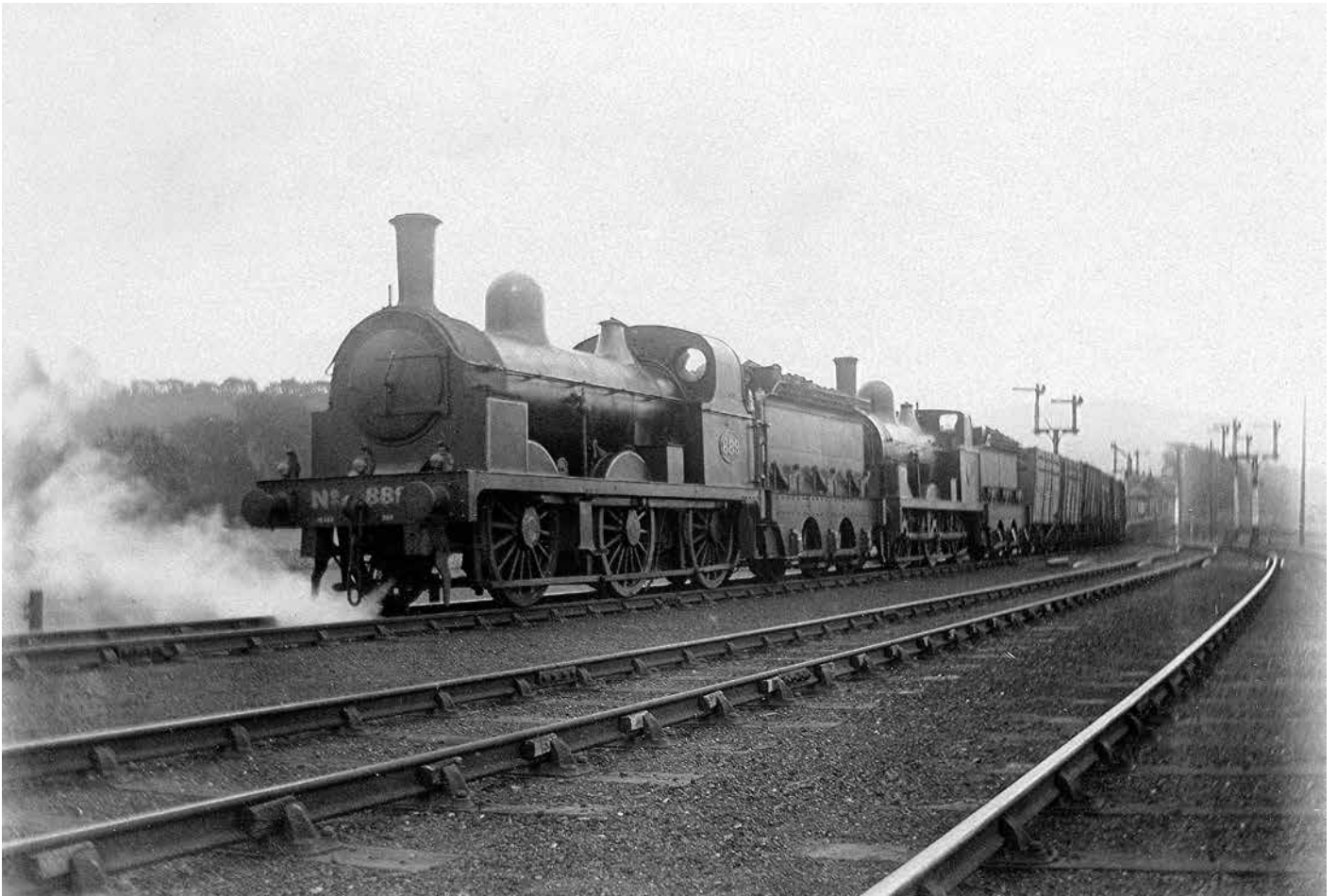
Kirkby Stephen probably about 1905. This image perfectly captures the essence of the double load coke trains. The locomotives Nos 889 and 670 are both members of the NER's 398 class. These seem to have replaced the 1001 class at Kirkby Stephen shed in the early years of the 20th century. The train itself appears to consist of a mixture of NER and privately-owned coke wagons.
